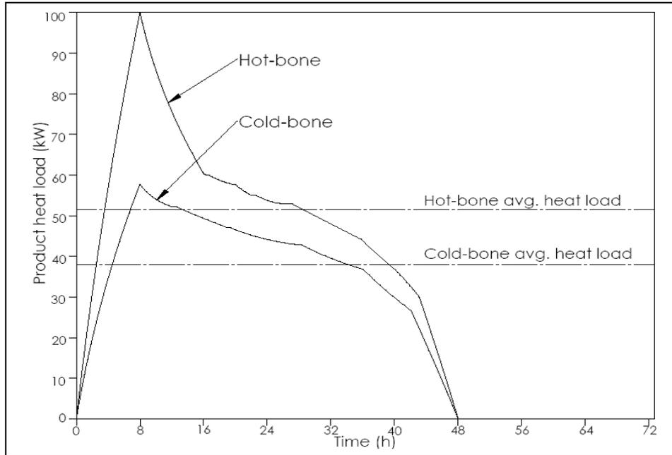
**Figure 7:** Product heat load characteristics for hot-boned and cold-boned beef cartons [47]
