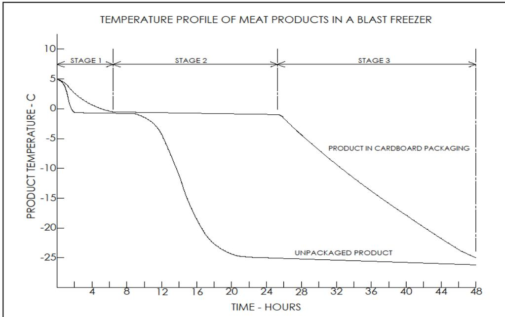
**Figure 4:** Freezing curves for packaged and unpackaged meat product in an air blast freezer
