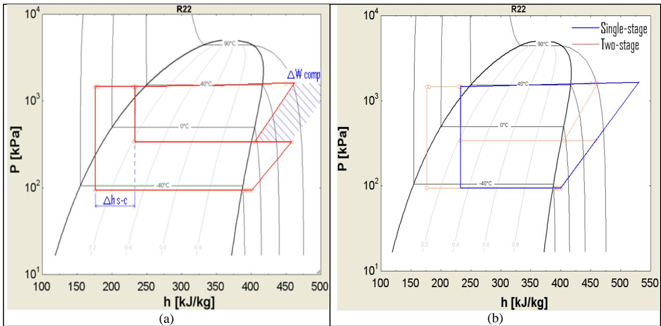
**Figure 6:** Two-stage P-h diagram from figure 5 system (a) and corresponding theoretical single stage P-h diagram operating with the same suction and discharge pressures (b)
