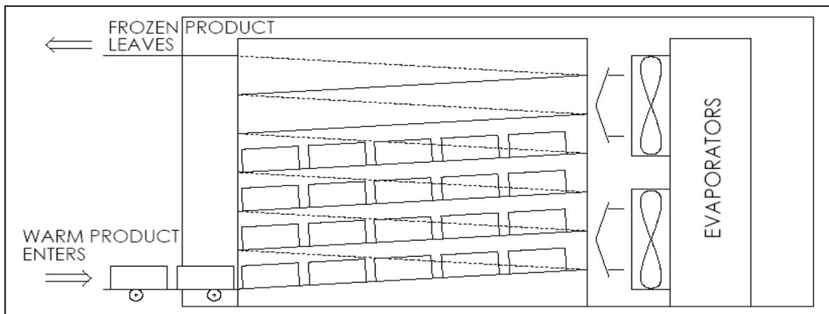
**Figure 2:** Schematic of a typical spiral Belt freezer
