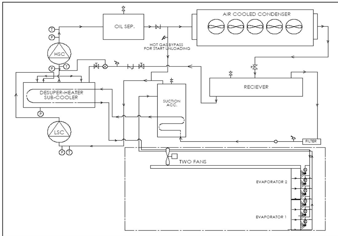
**Figure 5:** Schematic of a two stage carton blast freezer operating in New Zealand
