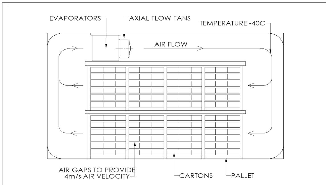
**Figure 1:** Schematic of a typical batch blast freezer
